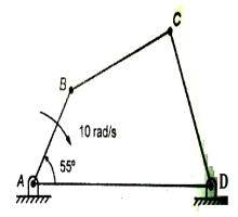
5. In a four bar chain ABCD, AD is fixed and is 150 mm long as shown in Fig.. The crank AB is 40 mm long and rotates at 120 r.p.m. clockwise, while the link CD = 80 mm oscillates about D. BC and AD are of equal length. Find the angular velocity of link CD when angle BAD =  $60^{\circ}$ .
